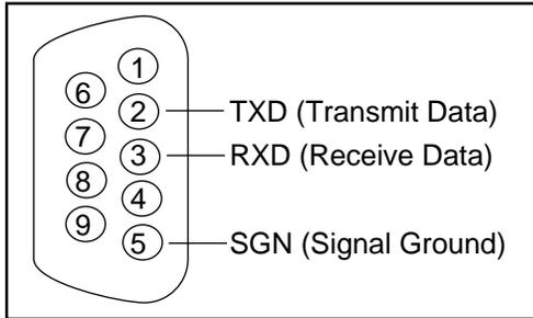
**Figure 5. RS232 (DB9) Connector**
