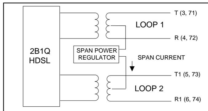
**Figure 2. HTU-C Span Powering Diagram**
