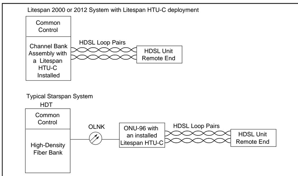
**Figure 3. Deployments from a Litespan Channel Bank Assembly**
