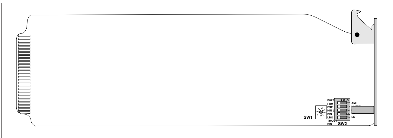
Figure 2. DDM Plus HTU-C Option Switch Locations
