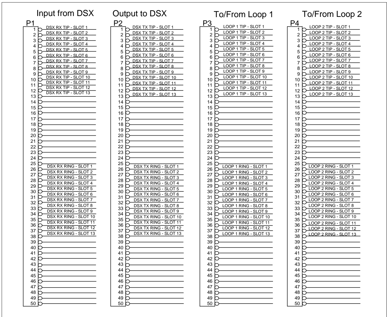
Figure 6. Signal I/O Pinouts for AMP-Type Connectors
