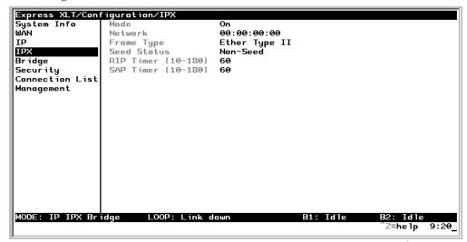
**Figure 3-5**Configuration/IPX Screen
