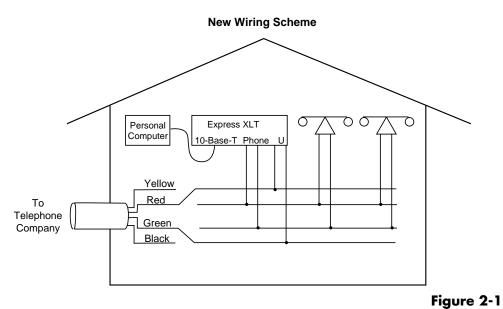
Wiring Scheme 1: Use existing analog telephone equipment, but replace single analog telephone service with ISDN service
