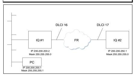
Figure 3-5. PC Connected to Local and Remote IQs
