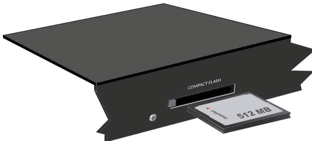
Figure 15. CompactFlash Card Installation
