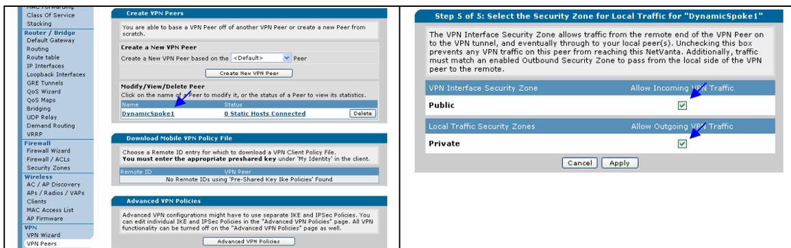
This type of firewall setup works for every Spoke. However, when the router has numerous VPN tunnels, there would be a firewall entry in each policy-class (Security Zone in GUI terminology) for each tunnel.
