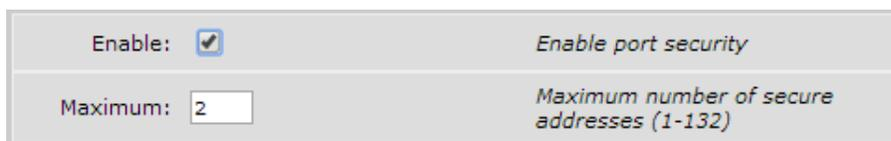
This screenshot shows a close-up of the configuration form. The 'Enable:' checkbox is now checked. Below it, the 'Maximum:' field contains the number '2'. The label for this field is 'Maximum number of secure addresses (1-132)'. The 'Enable port security' label is also visible above the checkbox.
