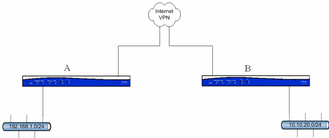
Above, there is a VPN that is established between 192.168.1.0 /24 and 10.10.20.0 /24. However, as time goes on, there may be a need for an extra subnet at each site to be accessible through the tunnel:
