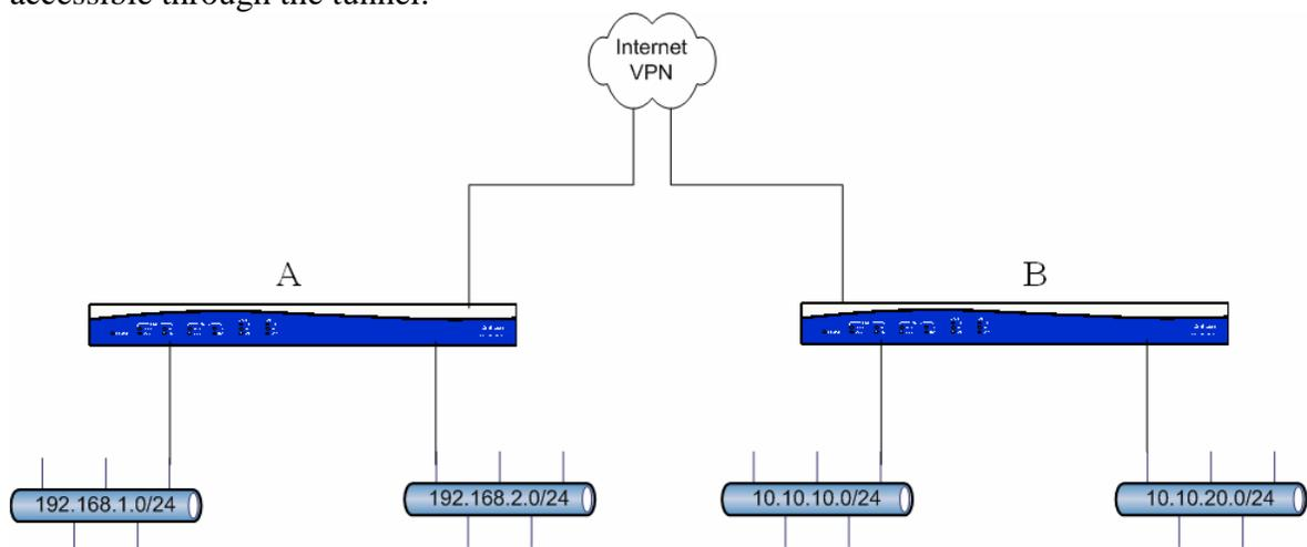
In this scenario, there are now two subnets on both sides that need to be able to reach the remote location. At this point, the selectors must be modified to add an additional subnet
