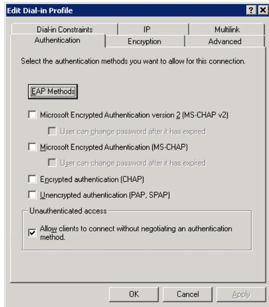
In the case of Port Authentication, an EAP method is used to authenticate. AOS currently only supports the use of the MD5-Challenge EAP method for Port Authentication. In IAS, it is done in the following manner:
