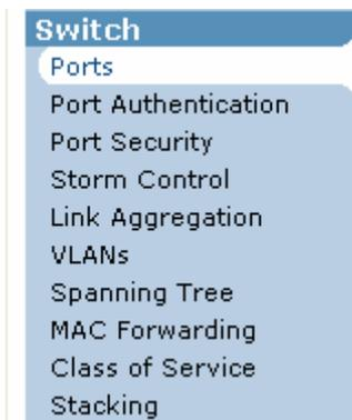
Once in this menu set the port to be used as a stacking port. It is important to note that this also puts the port into trunking mode, therefore there is not a need for another port to be configured for trunking.
