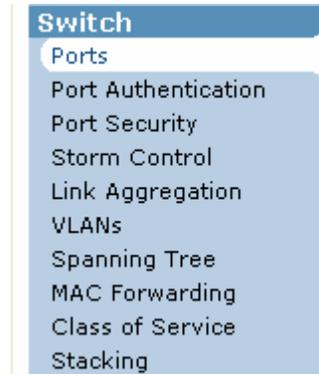
Once in this menu, set the port to be used as a stacking port to do stacking. It is important to note that if a port is assigned as a stacking port, it also acts as a trunk, therefore there is no need for an extra port for trunking..
