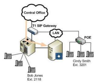
An external caller is routed through the PBX and terminates on an auto-attendant connected to the PBX (the UC server port connected to the PBX). The caller wants to dial Cindy Smith at extension 3201 on the UC server SIP PBX.
