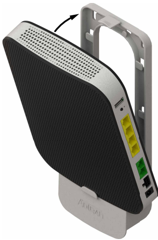
Figure 4. Attach ONT to ONT Fiber Tray and Bracket
