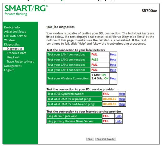
To refresh the data, click Test at the bottom of the page. The normal test method is initiated, utilizing OAM F5 loopback cells. The table is updated with fresh diagnostic information about connection integrity.
