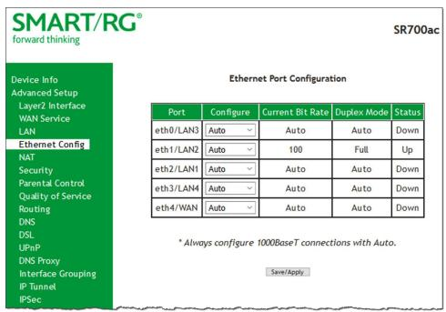
2. In the Configure column, select an option (Auto, 100 Full, 100 Half, 10 Full or 10 Half) for each of the four Ethernet ports on your gateway.
