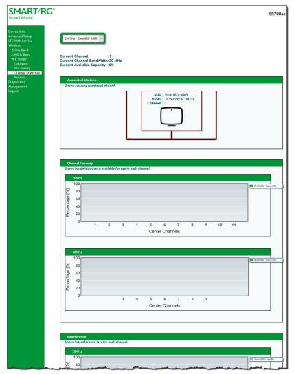
2. In the field at the top of the page, select the wireless band to review. Information is shown for associated stations, channel capacity, interference levels, adjacent channels, and channel distribution.
