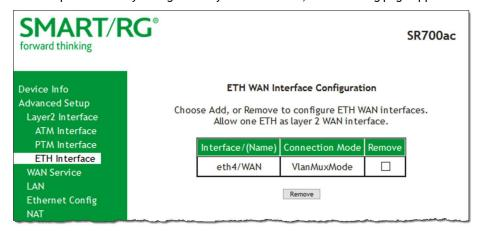
**Note:** If a WAN port it is already configured, you must remove it before you can define a new one. Before you can remove the existing port, you must first modify or delete any WAN service that uses it. The **Add** button does not appear until the existing port is removed.
