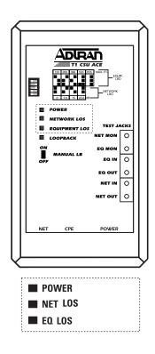
Figure 1-4. T1 CSU ACE LED Alarms
