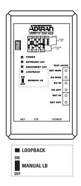
Figure 1-5. T1 CSU ACE Loopback Switch and LED
