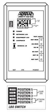
Figure 1-6. Line Build Out Switch
