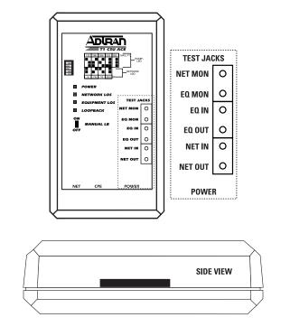
Figure 2-2. T1 CSU ACE Bantam Jacks
