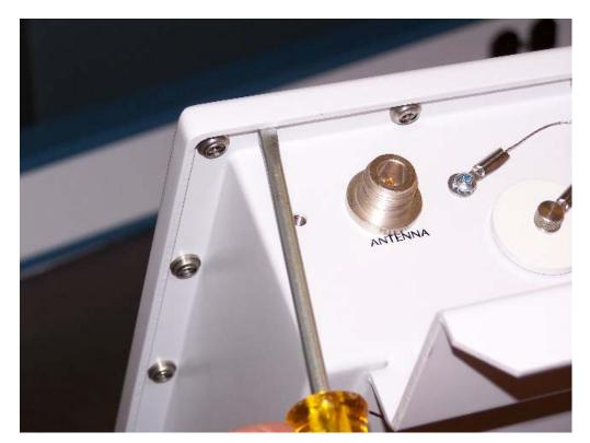
2. Insert flat blade screwdriver under corner of lid as shown.
