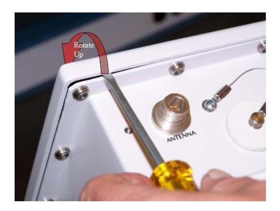
3. Gently pry up to break the seal of the weatherproof gasket.
