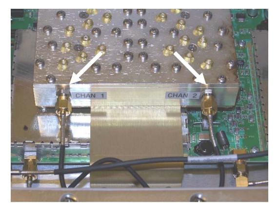
5. Remove TX and RX cables from the Diplexor and swap. Take care not to exceed a minimum bend radius of .750 in. Torque connectors to 8 in/lbs. If no torque wrench is available, tighten slightly more than finger tight. DO NOT overtighten!!
