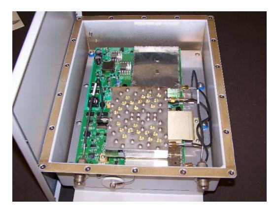
4. Remove lid and set aside. (Set as shown if safety lanyard is attached)
