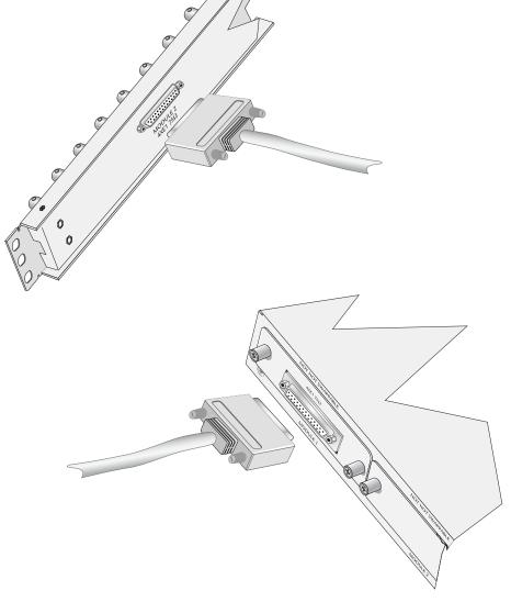
FIGURE 1. E1 CONNECTION WITH BREAKOUT PANEL
