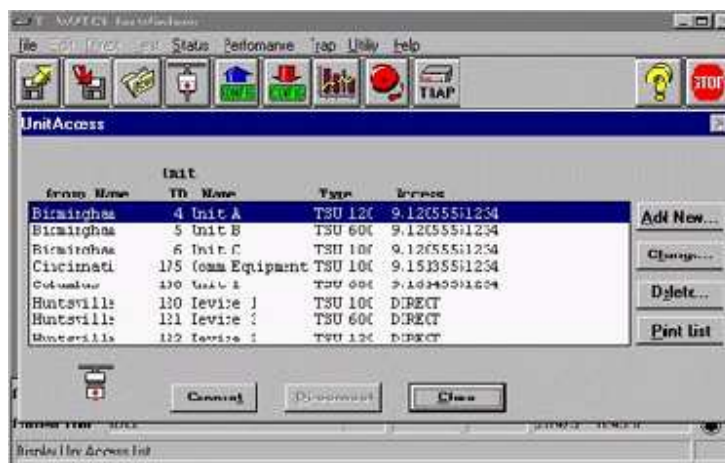
Figure 5: Select the unit with which to communicate in the Unit Access window
