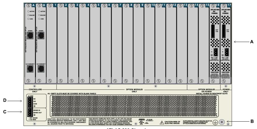
ATLAS 890 Chassis with 2 DC Power Supplies, 2 System Controllers, and 15 Blank Panels Installed
