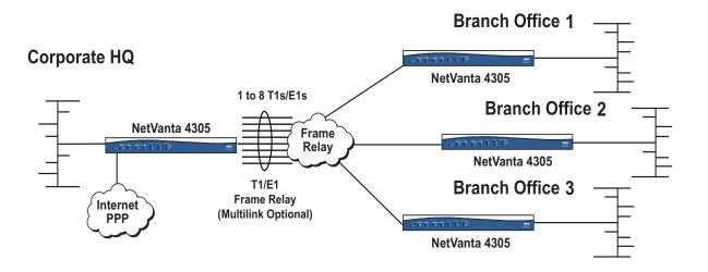
In the example network shown above, a corporate office provides centralized Internet access for three branch offices. Each branch is connected back to the corporate office using a Frame Relay link. The public Internet connection at the corporate office is provided using a point-to-point (PPP) connection to the Internet service provider (ISP). Refer to the following chart for configuration parameters required for this example.
