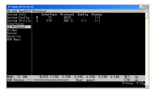
4. Arrow over to the Protocol column for the T1 interface. Hit Enter and select the appropriate protocol. For this example, we are setting up a PPP connection. When asked to confirm, hit Y.
