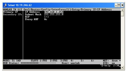
Note: If you are telnetting to the unit and you choose to change the Ethernet IP address, you will need to change the IP address of your workstation to an address on the same network as the Total Access to continue configuring the unit.
