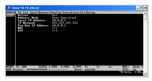
8. Return to the Router/Config/Interfaces menu and select Setup for the Ethernet interface. Select Primary IP and then enter the IP address that you have allocated from your LAN to be the routers IP address. Hit H to return to the main menu.
