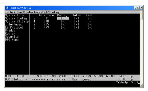
2. This is where you configure the frame format, line coding, and T1 timing. We are going to use ESF/B8ZS (which are the defaults). Now we need to set the T1 clocking. T1 clocking is extremely important. There can be one and only one clock source on a T1 circuit. In this example we are going to set the main side router to be the clocking for the T1 circuit. Set the Timing Mode to Internal.
