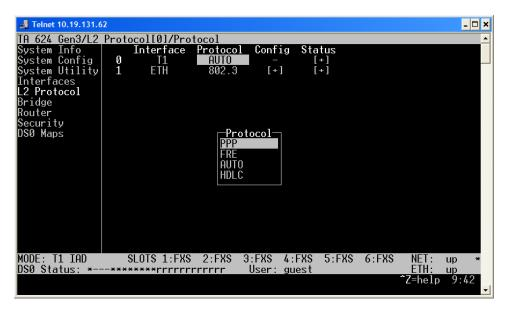
5. Arrow over to the Config column for the T1 interface. Hit Enter. Confirm that the Mode is set to Route IP as shown.
