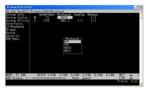
6. Arrow over to the Config column for the T1 interface. Hit Enter. Confirm that the Mode is set to Route IP as shown.
