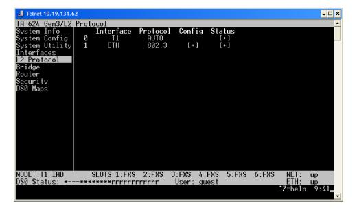
5. Arrow over to the Protocol column for the T1 interface. Hit Enter and select the appropriate protocol. For this example, we are setting up a PPP connection. When asked to confirm, hit Y.
