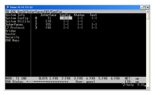
2. This is where you configure the frame format, line coding, and T1 timing. We are going to use ESF/B8ZS (which are the defaults). Now we need to set the T1 clocking. T1 clocking is extremely important. There can be one and only one clock source on a T1 circuit. In this example we are
