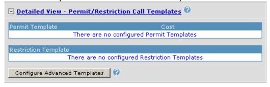
Add an appropriate entry by configuring the 'Template' and 'Cost' according to your call routing strategy. In this case, all calls will be routed out of the SIP trunk so the Template should be '\$' and the Cost should be '0'. When finished, click on the 'Add' button.
