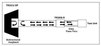
Figure 6. TROCU DP Bidirectional Loopback
