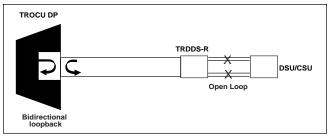
Figure 7. TROCU DP Bidirectional Loopback
